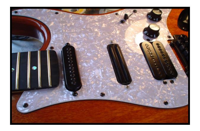
This rial pickup uses the same color codes as a Gibson pickup. Red is hot, black is ground, green and white form the series link, and the bare wire also goes to ground.
